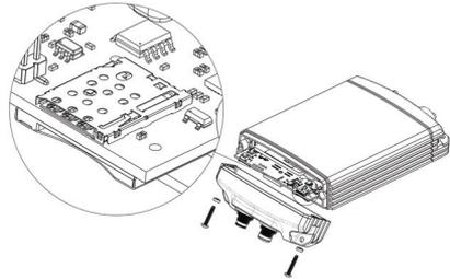
Insert the Iridium and cellular SIM cards in the slots behind the connectivity port (the Iridium SIM slot is the larger of the two slots). Re-attach the bottom panel and tighten the screws, taking care not to damage the cable wires.
