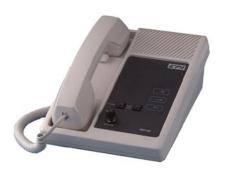
The RST300/PST300 remote system allows fixed site users access to the transmit and receive functions of the G2 unit from any 2 wire voice grade pair. This allows in building operation away from the main G2 unit and in areas where antenna placement may be a problem. All parallel remotes receive all incoming and outgoing audio as well as provide LED indicators of the G2 status indicators.
