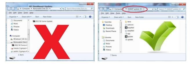
Apply power to the message terminal allowing the easyMail application to start up, then close the easyMail application. Go to Start >My Computer > and double click on the Data (D :) drive, then open the folder named "easyMailData". Then open the folder named "html", and delete all the files in this folder, then close this window.
