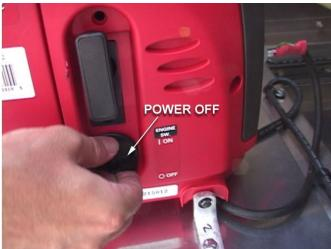
POWERING OFF – Make sure to turn off the Electronics power BEFORE you turn off the generator. This will help protect the electronics from any electrical fluctuation.
