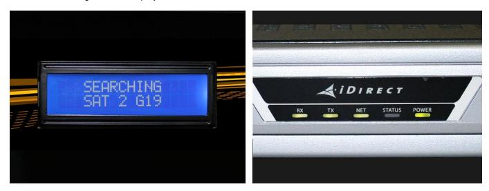
The TS2 will show the current status of the system. When the iDirect X5 Router LED lights turn green (only the Status light should be dark), you are online. If the power light on the X5 is solid green and the TX light is blinking green, the system is still acquiring the satellite.
