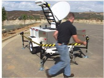
**STEP 12 – RETRACT THE SECURITY BELT** - The T-100 has two retracting security belts that keep foot traffic from accidentally bumping the trailer, and from standing too close to the transmitter.
