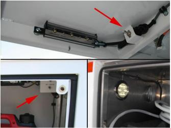
**STEP 8 – OPEN THE GENERATOR CABINET**. If dark, you may use the toggle switches for cabinet lights as well as emergency flashers, both of which may run on internal battery. The rear bay has a single switch to turn on the bay lights. The generator may say in the cabinet (running with door open), or removed from the cabinet.
