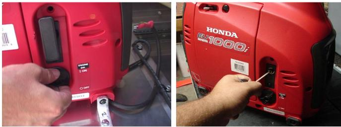
Turn on the POWER Switch to ON, and then firmly and quickly pull the starter cord to start the generator. IMPORTANT - Make sure to turn off the choke after the motor has started.
