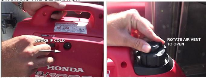
STEP 9. START THE GENERATOR. Close the choke if the generator is cold and open the air vent on the gas cap.
