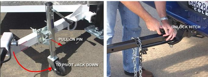
**STEP 3** – Pull the pin the holds the front wheel jack against the trailer frame. Rotate it 90 degrees so that the jack locks into place with the wheel side down. Carefully unlock the hitch from the ball.
