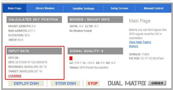
First, look to the lower left quadrant of the screen, to the "Input Data" Section: Confirm that it displays "GPS Signal OK" and has GPS coordinates. When GPS is "OK", you may click on "Deploy Dish". This dish will lock on satellite and create an Internet connection automatically.
