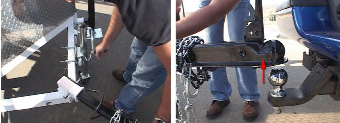
STEP 4 - Begin to crank up the front of the trailer so that the hitch clears the 2" ball on the tow vehicle.
