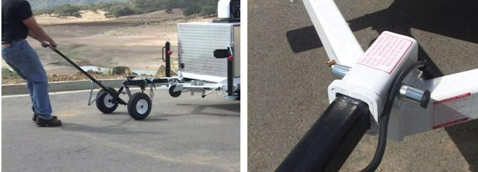
The trailer dolly is a good way of moving the trailer to a different location. Also note the trailer tongue itself may be removed by unlocking the locking pin that holds it to the trailer frame. Removing the tongue may reduce theft of the system, or allow other tongue configurations to quickly be used on the trailer.
