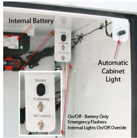
An onboard battery powers cabinet lights and the trailer's emergency flashes when the generator is not running. Helpful for dark nights.
