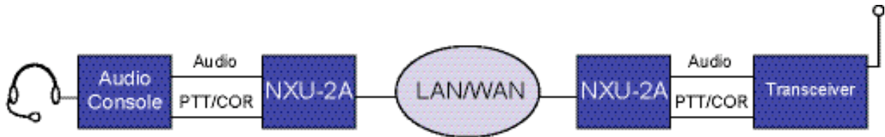
Figure 2. Illustrates a basic NXU-2A application in which a communications transceiver is connected via a network to a remote audio console. The transmit/receive audio and the PTT/COR signals are transported digitally across the network and appear transparently at the other end. The operator at the audio console can use the radio as if it were located right beside him.
