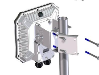
6. When LED flashes yellow: Turn and tilt the EXPLORER 540 and use the pointing sound to obtain the highest possible signal strength. (continuous sound = best signal)
