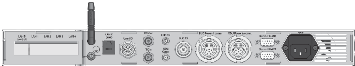
Figure 4-3: ACU rack version, connector panel overview
