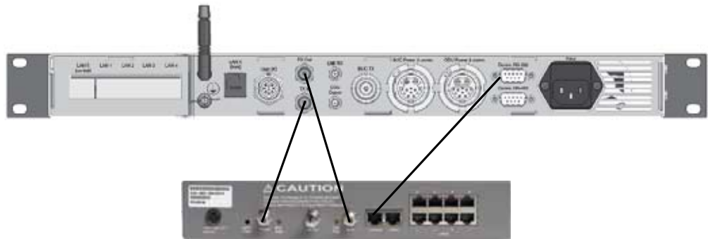
Figure C-7: Connecting iDirect iNFINITI 5000 series to the ACU (Serial)
