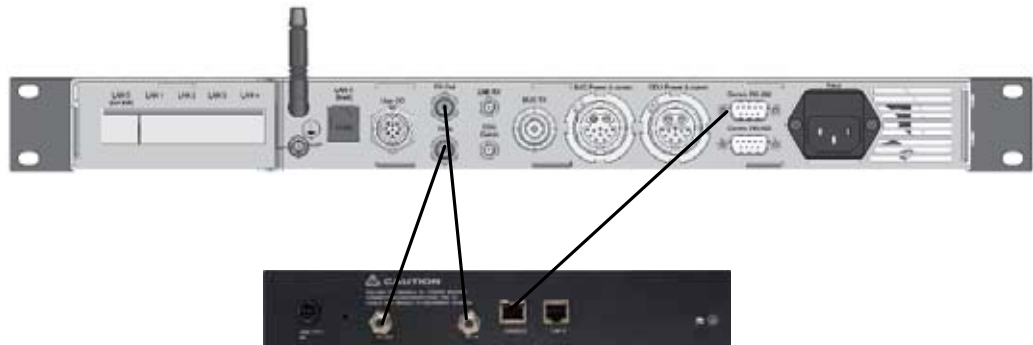
Figure C-8: Connecting iDirect Evolution X5 to the ACU (Serial)
