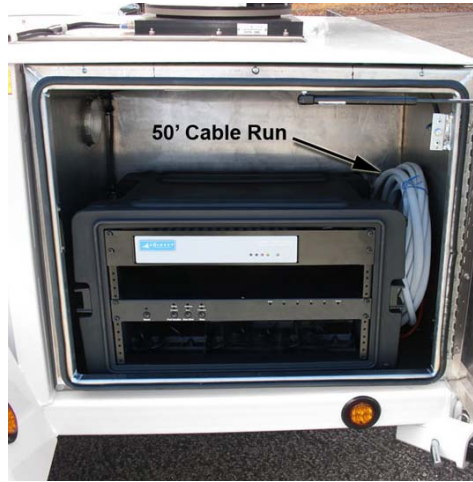
A 6RU rackmount case is locked behind a stainless steel weather-proofed trailer cabinet door. The rack-mount itself can be moved up to 50 feet from the trailer, and placed inside of a structure or tent if desired.
