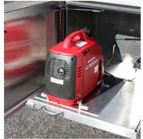
The 1000W Honda ultra-quiet generator is more than capable of handling the 90 Watts the system pulls at maximum power. It can run for more than 8 hours on a single tank (one gallon) of gas.
