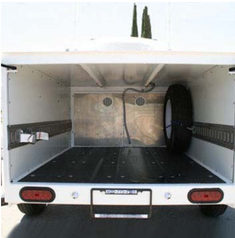
The weather resistant enclosed rear lockable storage bay includes a spare tire. Interior dimensions are 62"L x 46"W x 24"H.
