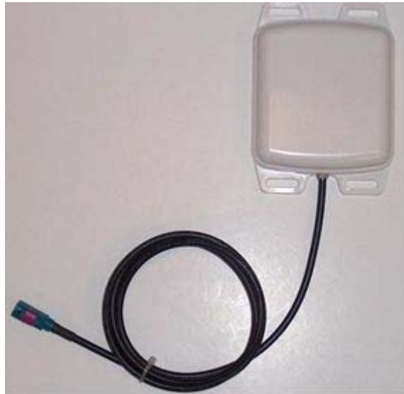
Figure 5 Satellite/GPS Side Entry Antenna
