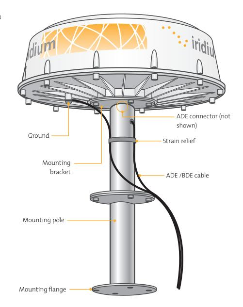
**Note:** The mounting configuration may vary depending on the factors discussed (e.g.: location, pole selection). When mounting the bracket ensure:
