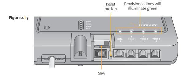
The handsets connected to the BDE must be POTS / RJ11 handsets. The data port provides an Ethernet connection of 10BaseT/100BaseT using an RJ45 connector connected as MDI-X. If the Below Decks Equipment (BDE) is to be connected to a down-stream port of an Ethernet hub or switch then the user will need to use a cross-over cable. Again, the data port must be provisioned to connect to the Internet. The data LED will illuminate green.
