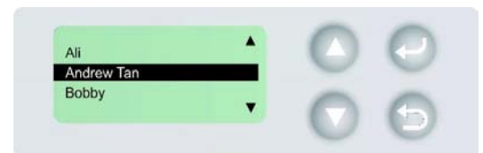
FIGURE 4.4.1-3: LCD Display of SABRE™ I showing the contents of the Phonebook.
