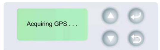
FIGURE 3.6.3-1: LCD display indicating that SABRE™ I is acquiring a New GPS Fix.
