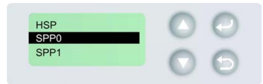
FIGURE 4.3.3-1: LCD Display of SABRE™ I showing the selection of the "SPP0" profile from the list of available profiles that are supported by the Bluetooth Dongle.
