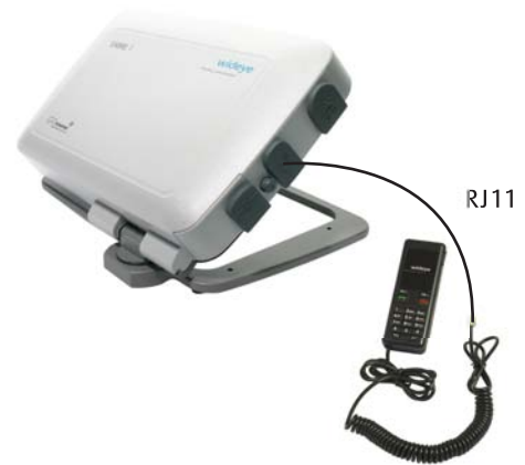
FIGURE 4.1.1-1: Figure showing the connection of the Corded Analog Handset to the RJ-11 Interface of SABRE™ I.
