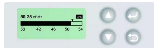
FIGURE 3.6.3-5: LCD display indicating the Signal Strength Bar
