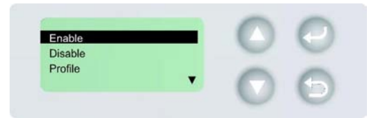
FIGURE 4.3.1-1: LCD Display of SABRE™ I showing the Bluetooth Interface “Enable” Option screen.
