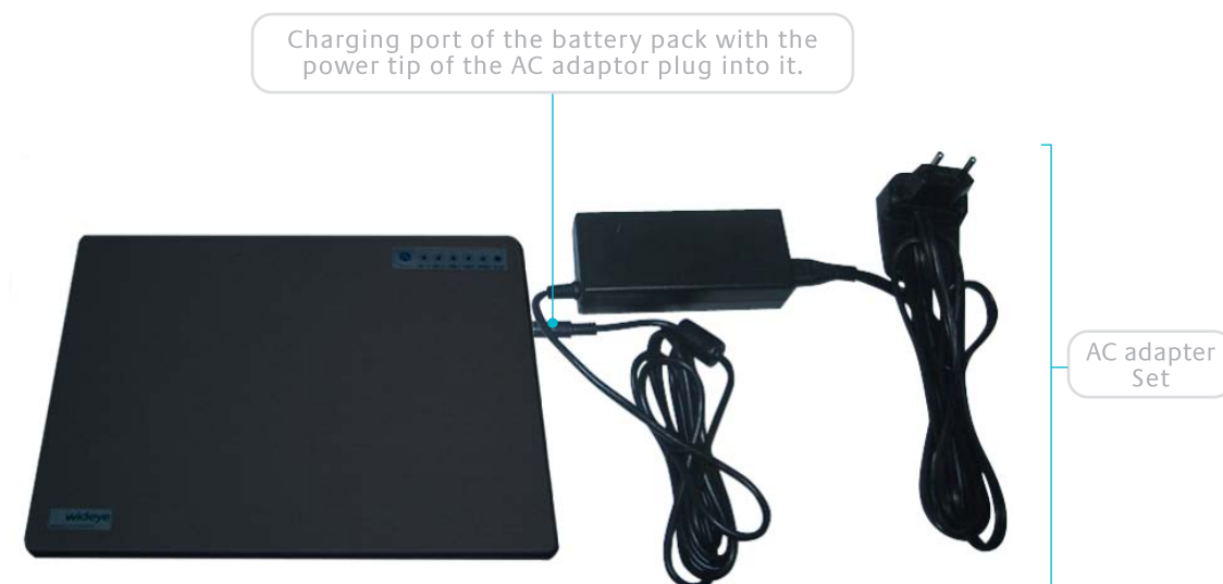
FIGURE 5.5-2: Setup for charging the Secondary Battery Pack
