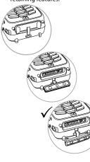
2. Press down the latch button and then gently rotate it up to open the latch. Place the Iridium Extreme handset into the PotsDOCK Extreme.
