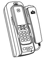
Privacy Handset mode is enabled when the handset is removed from the cup. Please ensure to re-dock the Privacy Handset when not in use.
