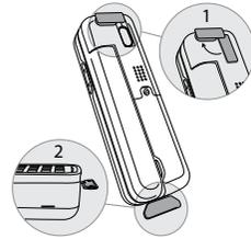
3. To dock the handset, align the IsatPhone with the phone tray and slide the handset down until it seats flush to the bottom of the tray. Swing the phone down into the cradle by applying pressure to the top of the handset. An audible ‘click’ is heard when the phone is in the docked position.
