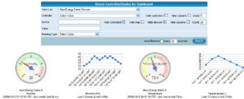
After logging into the system the Dashboard page will be the first page presented. The dashboard will display any widgets created to monitor your sensors/equipment and a map if your controller has the optional GPS. The map will display the last location reading sent into the system.
