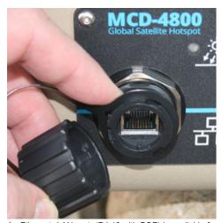
An Ethernet LAN port (RJ-45 with POE) is available for a hard wire Internet connections. Normally it is capped sealed when not in use. The panel display shows battery life and the temperature of internal electronics.
