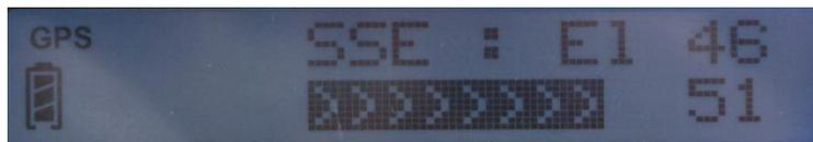
Use the signal quality bar and numeric display on the lower line to help point the UT to the satellite. While in pointing mode, you may also activate the audio pointing aid by a long press of the audio button on the right.
