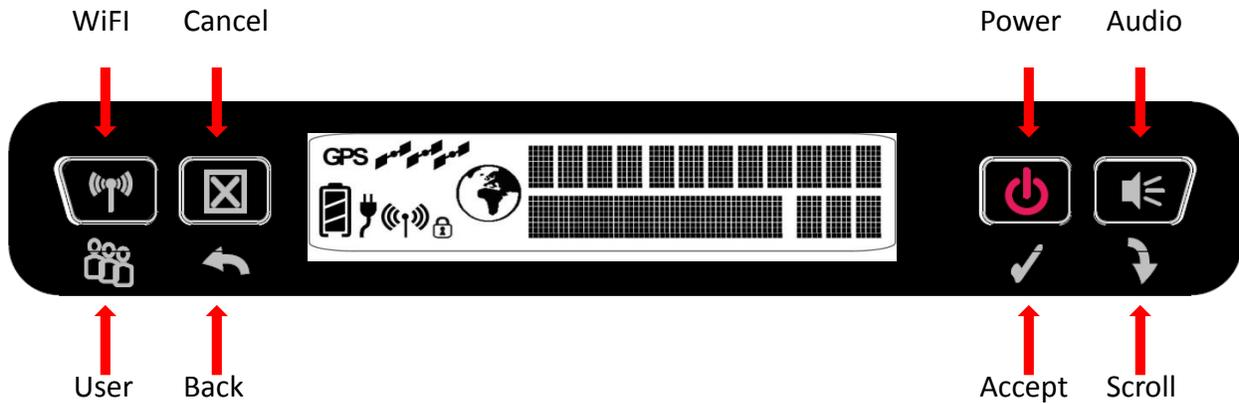
The top line gives the compass bearing and elevation angle of the closest satellite.
