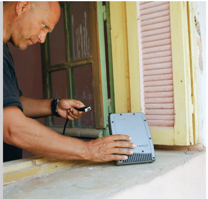
Connecting Antenna Unit of the Nera WorldPro 1000 for indoor use.
