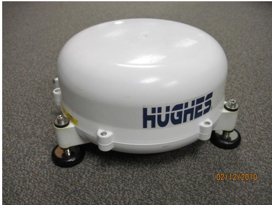
Figure 8. C11 antenna ODU 252 mm x 119 mm height
